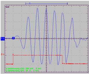
The oscilloscope plot above shows the R-1 Rototactor responding to a short 29 ms, 10 volt pulse, i.e. the red line. The blue line shows the pressure wave generated by the Rototactor in a standard skin and flesh simulator. Note the 10 ms response time and the sinusoidal tactile signal waveform. Also note the 200 Hz vibration frequency, and the signal strength of 1.3 Ruperts peakto-peak, delivered by a tactor weighing just 2 grams.
