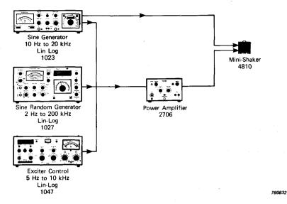
Fig.2.1. B & K Exciter Control Generators and Power Amplifiers for use with the 4810 Mini-Shaker
