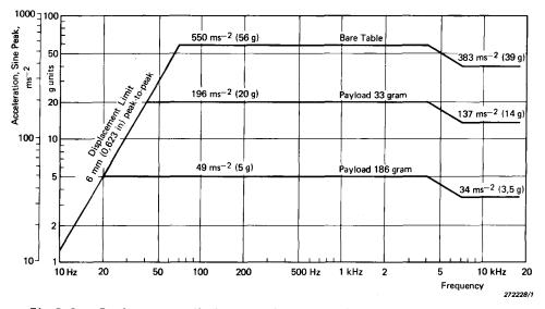
Fig.3.3. Performance limits for sine operation of the 4810 Mini-Shaker
