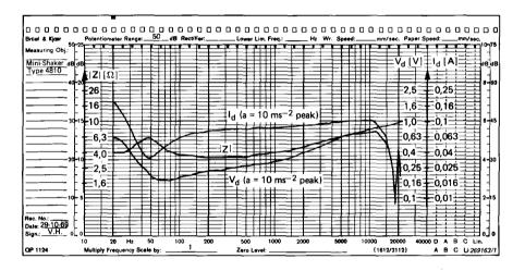
Fig.3.2. Typical frequency response of the 4810 Mini-Shaker
