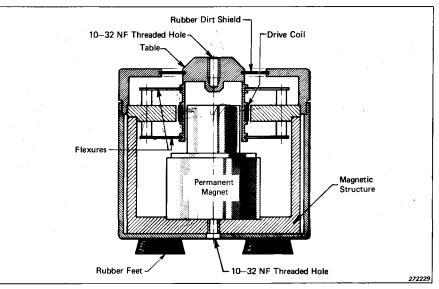
Fig.1. Sectional drawing of the Mini-Shaker Type 4810
